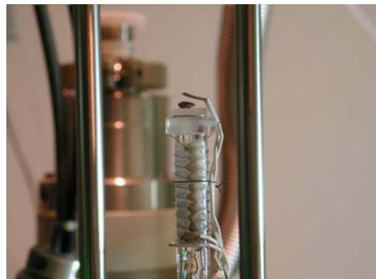
Fig. 1 Setting of Si on SiO 2 substrate; thermo-couple is located above Si
