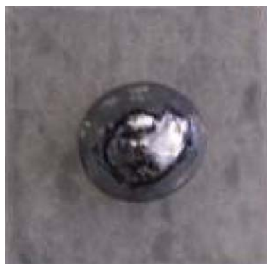
Fig. 7 Si droplet on BN substrate after cooling: Si droplet did not move at all under 20 Torr with Ar flow of 2 L/min and the BN substrate was not colored, as revealed in Fig. 4
